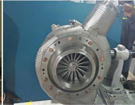
Turbocharger for T-92 tanks
